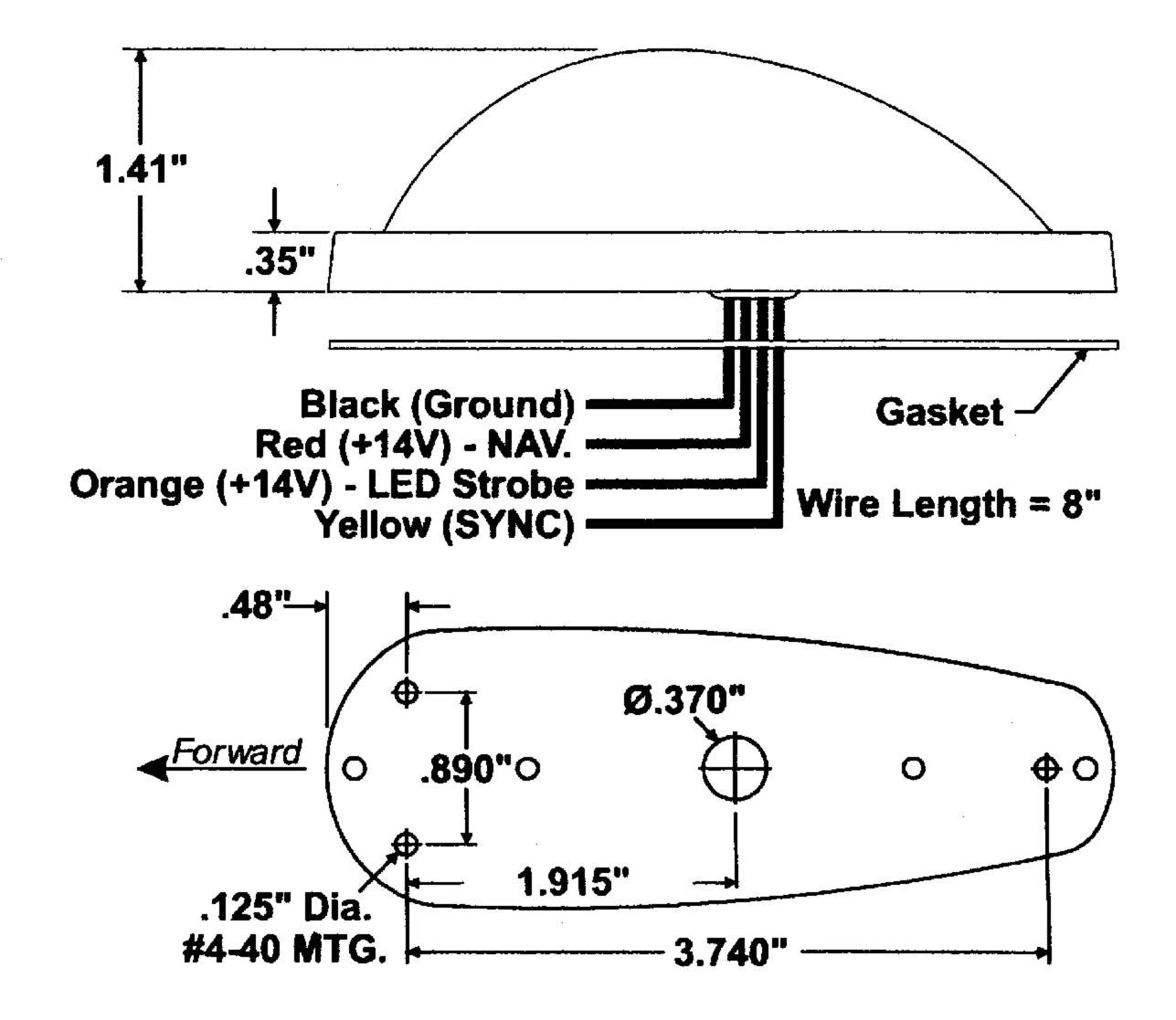
NOTE: Connecting the SYNC (Yellow) wires together will cause those lights to flash at the same time. If synchronization is not necessary or desired, the connection may be left open.
